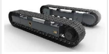
A bracketed frame with machined plates provide a simple bolt on interface reducing assembly time. Standard bracketed models are available in many sizes.
