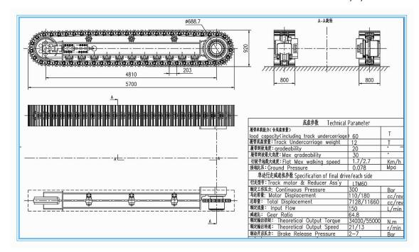
Dimension can be customized (length A, width of track shoe E, height C)
