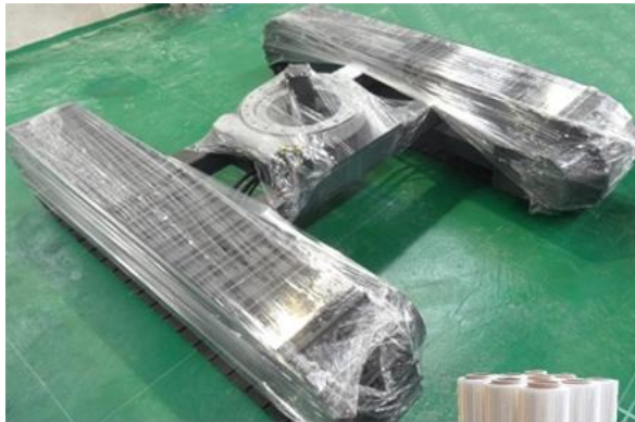
1.Wrap the undercarriage with wrapping film
